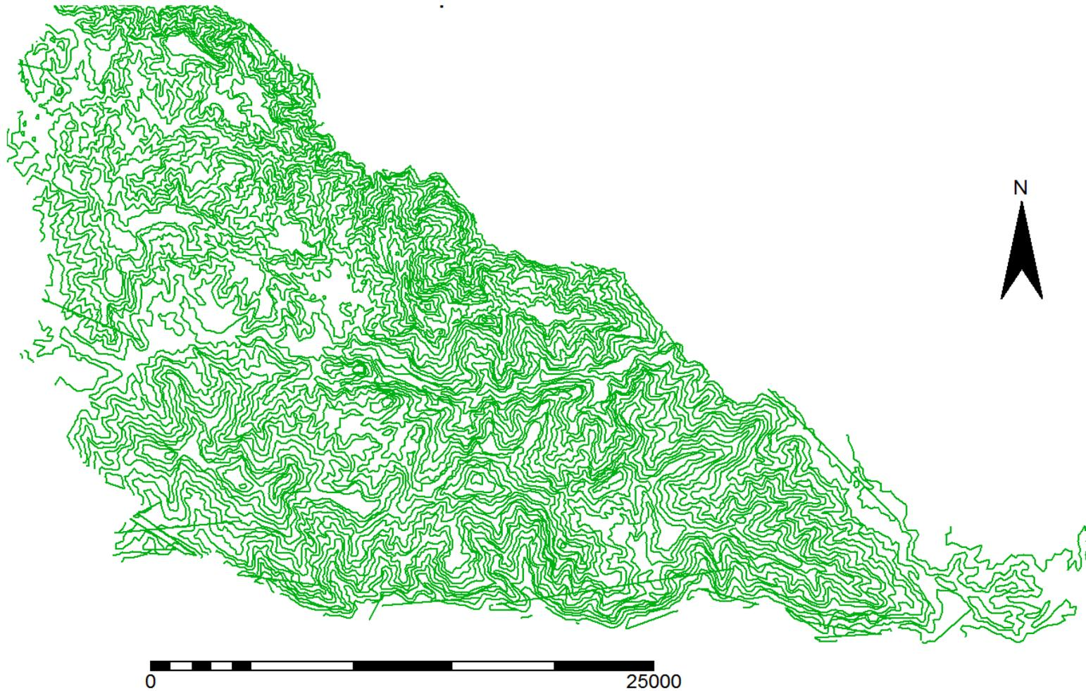
Map 3. Contour map of Irobland with the contour interval (spacing) of 50 meters
