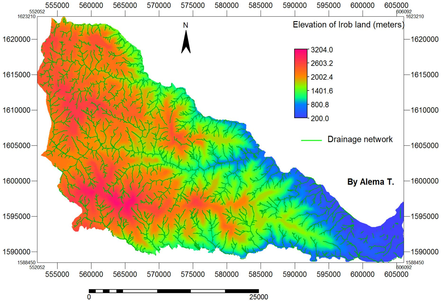
Map 5. Drainage systems superimposed on Digital Elevation Model (Elevation map) of the Irobland
